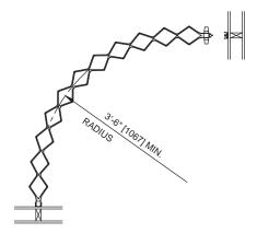
**CURVED TRACK/RADIUS CONSTRUCTION** #4 track can be custom made to fit almost any curve of at least 3'-6" [1067] radius. Accordion doors with optional radius construction can follow curves and straight track.
