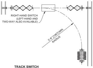
Accordion doors with radius construction can be stacked in remote locations by using single or two-way track switches.
