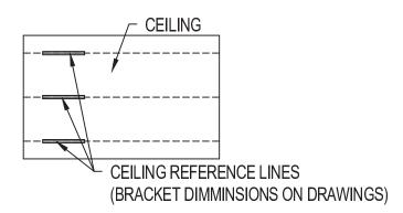
3. SECURE THE EC-2 BRACKET / EC-4 BAR TO THE CEILING WITH SCREWS.
