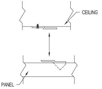
\*APPLY A SMALL AMOUNT OF ADHESIVE ON BOTH PARTS OF THE BRACKETS. THEN SLIDE BRACKET TOGETHER
