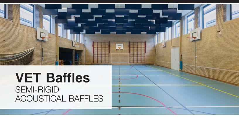
Semi-Rigid VET Baffles are the perfect economical solution to reverberation issues for large spaces. They are easy to install suspended down from the ceiling via grommets. The VET Baffles are all custom made with a wide variety of finishes and sizes available.
