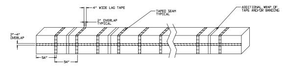
Stick pins / weld pins to be utilized every 12" - 18" depending on duct size and installer reccomendations (Bottom of Duct Shown)
